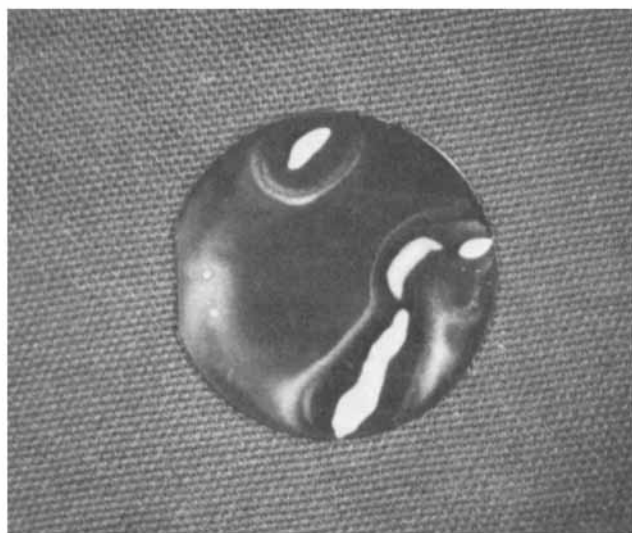
Fig. 11. Slice cleaned at 1,200°C with HCl, exposed to air, and 998°C H 2 -etched before deposition of 3 μm layer.
